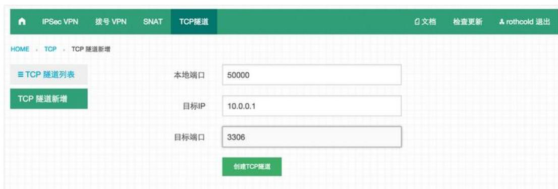
The screenshot shows the 'TCP Tunnel' management interface. On the left, there are navigation options: 'TCP Tunnel List' and 'Add TCP Tunnel'. The main area contains three input fields: 'Local Port' with the value 50000, 'Target IP' with the value 10.0.0.1, and 'Target Port' with the value 3306. Below these fields is a green button labeled 'Create TCP Tunnel'.
